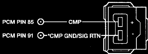
CAMSHAFT POSITION (CMP) SENSOR HARNESS CONNECTOR VARIABLE RELUCTANCE
