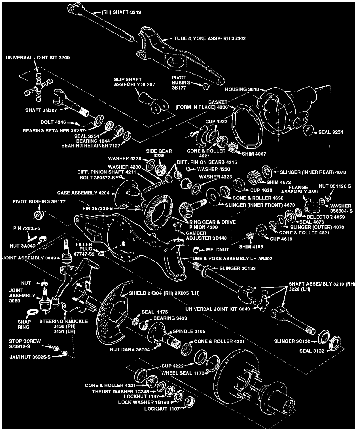
Fig. 4 Disassembled view of Dana/Spicer model 50-1FS front drive axle
