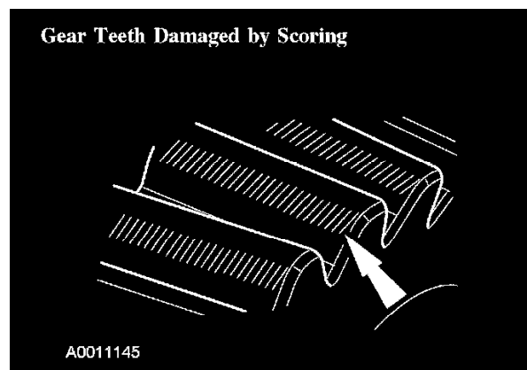
Gear Teeth Damaged by Scoring
