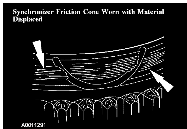
Synchronizer Friction Cone Worn with Material Displaced
