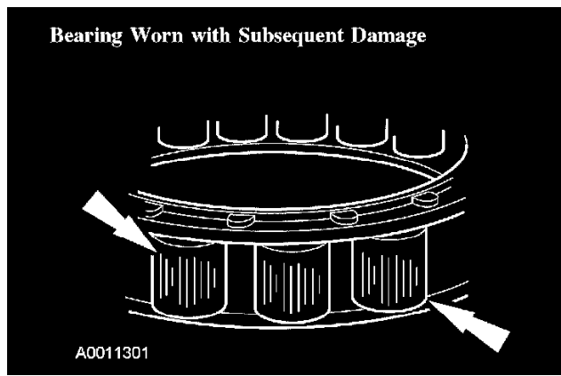
Bearing Worn with Subsequent Damage
