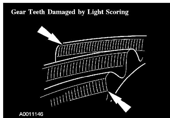
Gear Teeth Damaged by Light Scoring
