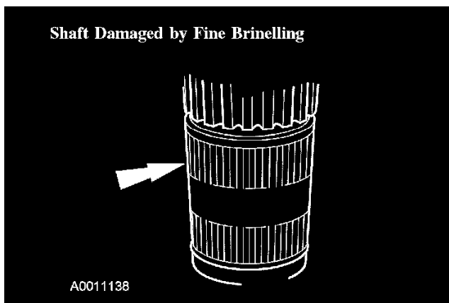
Shaft Damaged by Fine Brinelling
