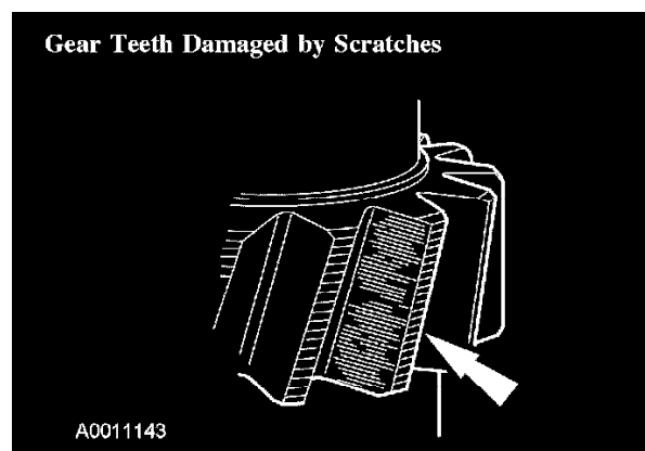
Gear Teeth Damaged by Scratches
