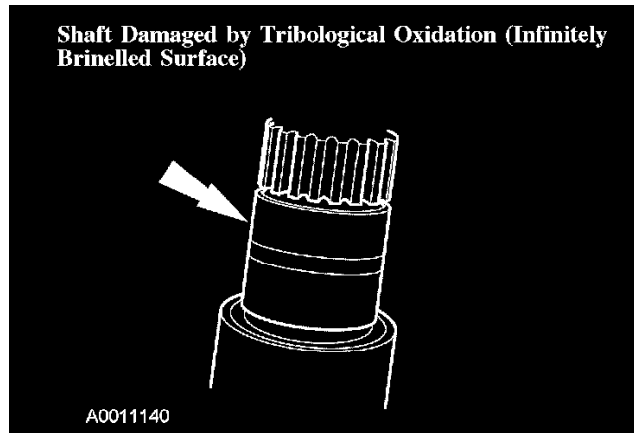
Shaft Damaged by Tribological Oxidation (Infinitely Brinelled Surface)
