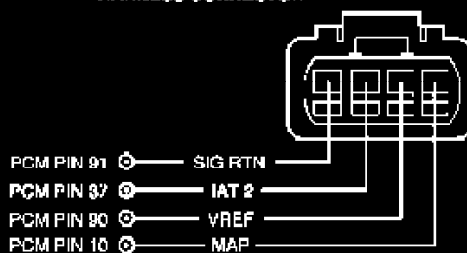
THERMAL MANIFOLD ABSOLUTE PRESSURE (TMAP) SENSOR HARNESS CONNECTOR
