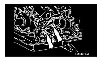
8. Remove the three bolts, the nut and the oil filter adapter.
