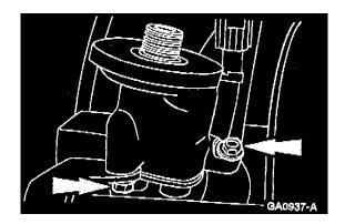
7. Remove the bolts, and remove the remote oil filter adapter.
