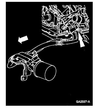
5. Remove the two nuts and disconnect the remote oil filter adapter.
