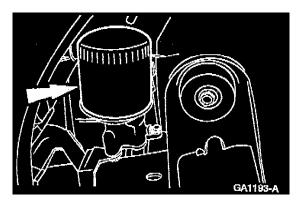
6. Remove the oil bypass filter.
