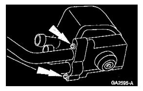
3. If equipped with an oil cooler, remove the two nuts and disconnect the remote oil filter adapter from the oil cooler.
