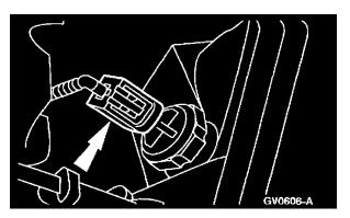
4. If the vehicle is not equipped with an oil cooler disconnect the oil pressure sender electrical connector.
