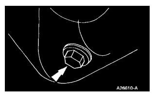
2. Remove the drain plug and drain the engine oil.
